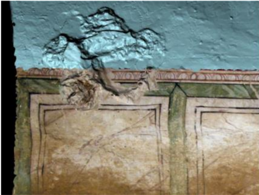
Photo overlay in visible with the intensity distribution map for laser-induced fluorescence scanning
